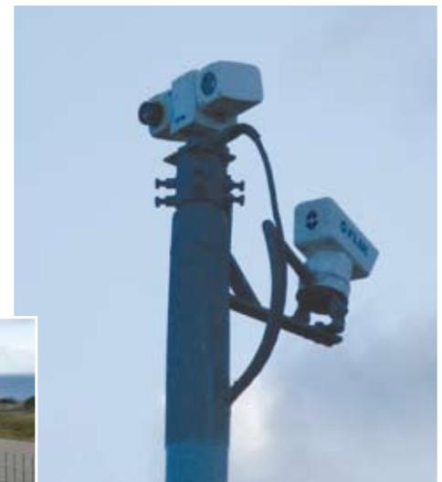
A PatrollIR and PTZ-50 MS mounted together on a mast to secure the perimeter
