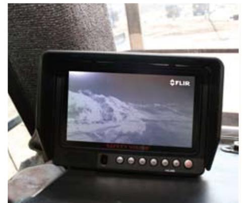
*The thermal images produced by the PathFindIR are displayed on a large LCD display inside the trucks cabin. They help the driver to avoid accidents.*
